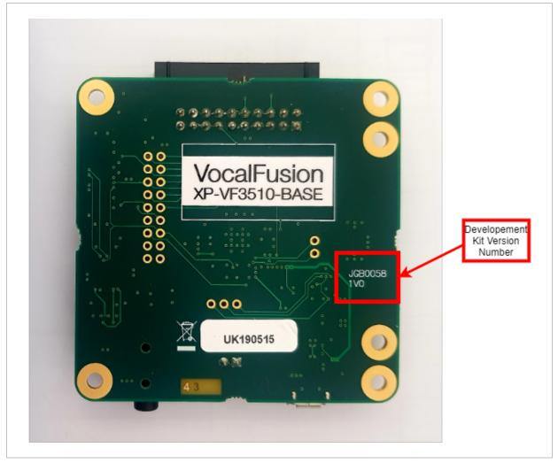
Figure 2-2 Version number location on the underside of XVF3510 Processor Base Board
