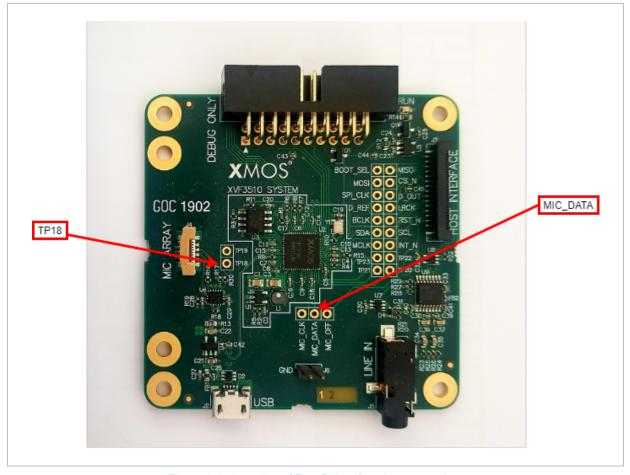
Figure 3-1 Location of Test Points for wire connection.
