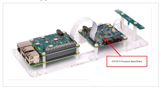
Figure 2-1 Location of XVF3510 Processor Base Board
