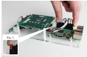
This cable provides I<sup>2</sup>S digital audio and I<sup>2</sup>C control
