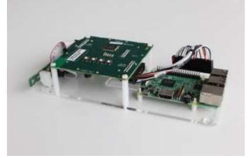
Secure the Pi with the supplied plastic nuts (optional)
