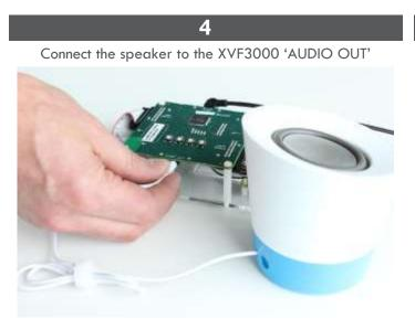
Place the speaker adjacent to and behind the mic array Note: only the left channel is active, right is muted
