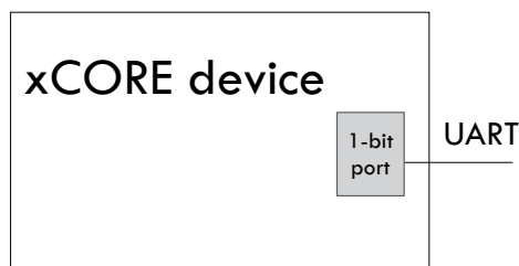
Figure 3: UART half duplex connection
