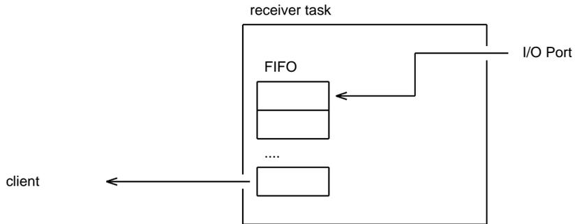
Buffering data in this way decouples the client task from the receiver so that the client is not bound by the real time constraints of the I/O.
