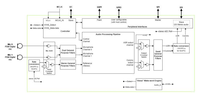
Fig. 2.3: Functional block diagram of XVF3615 in INT configuration
