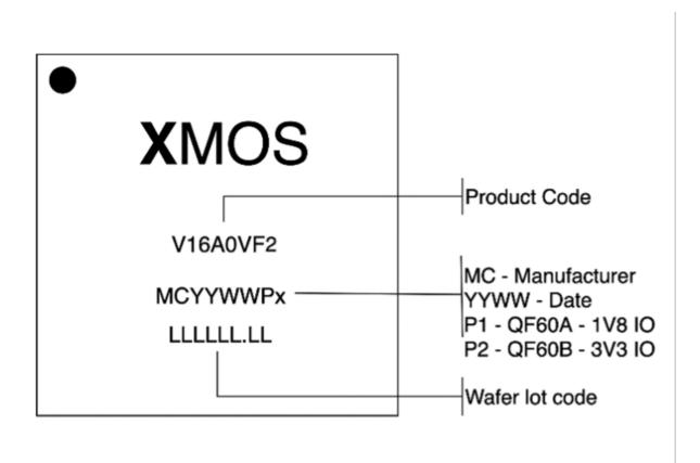
**Important:** The picture above represents the commercial package, the industrial package is distinguished by an *I* after the product code, i.e. V16A0VF2I.
