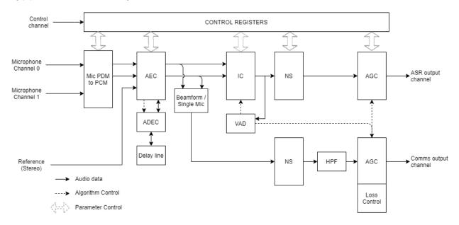
Fig. 3.1: The XVF3615 audio processing pipeline
