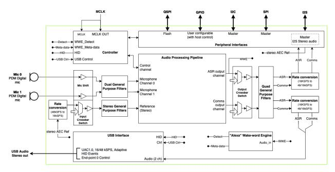
Fig. 2.2: Functional block diagram of XVF3615 in UA-HYBRID configuration
