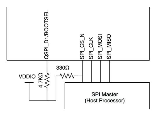
Fig. 5.2: XVF3615 SPI Slave boot configuration
