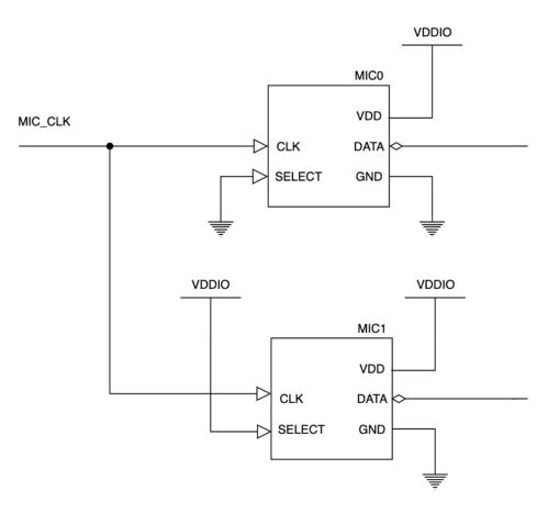
Fig. 5.1: PDM microphone schematic
