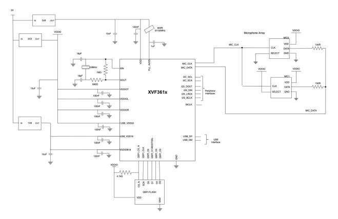
The essential components and signals for a XVF3615-UA application with 3V3 I/0 is shown in the figure below.
