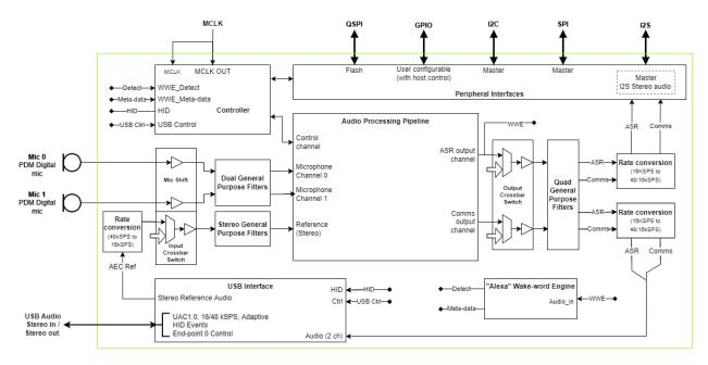
Fig. 2.1: Functional block diagram of XVF3615 in UA configuration
