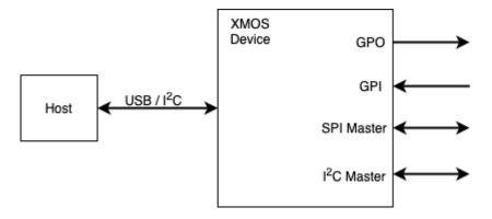
Fig. 3.1: Device GPIO interfaces
