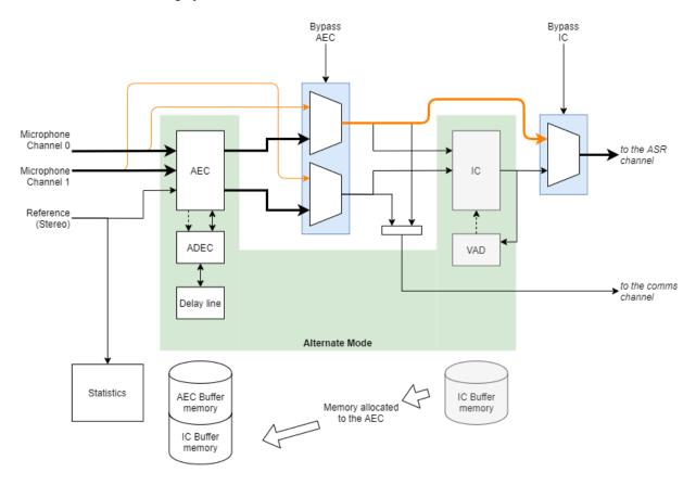
Fig. 2.9: Audio pipeline configuration, [ALT\_ARCH=1] when reference signal is present
