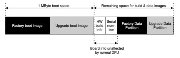
Fig. 4.1: Flash data structure for VocalFusion® XVF3610
