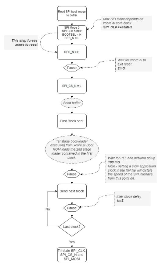
Fig. 4.2: SPI Boot process and timing requirements
