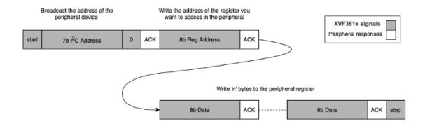
Fig. 3.4: I<sup>2</sup>C protocol for register writes
