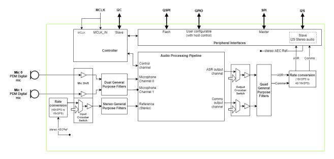
Fig. 1.3: Functional block diagram of XVF3610 in INT configuration
