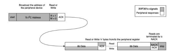
Fig. 3.5: I<sup>2</sup>C protocol for raw reads and writes
