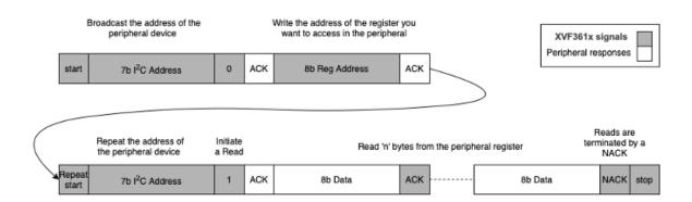
Fig. 3.3: I<sup>2</sup>C protocol for register reads
