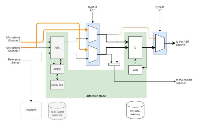
Fig. 2.10: Audio pipeline configuration, [ALT\_ARCH=1] when reference signal is absent
