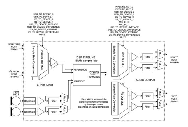
Fig. 2.1: XVF3610 input, output and audio signal routing
