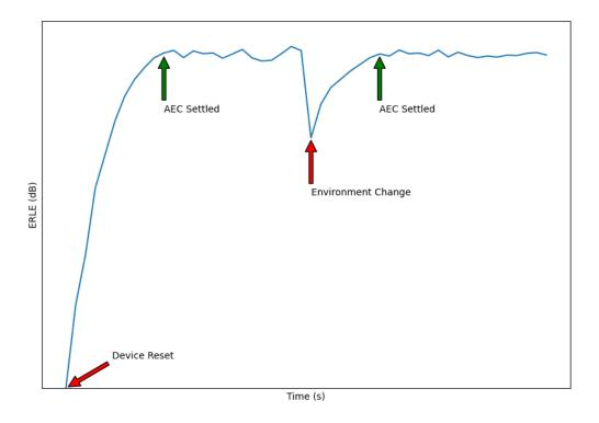
Fig. 2.5: Settling time of the AEC shown using an ERLE plot
