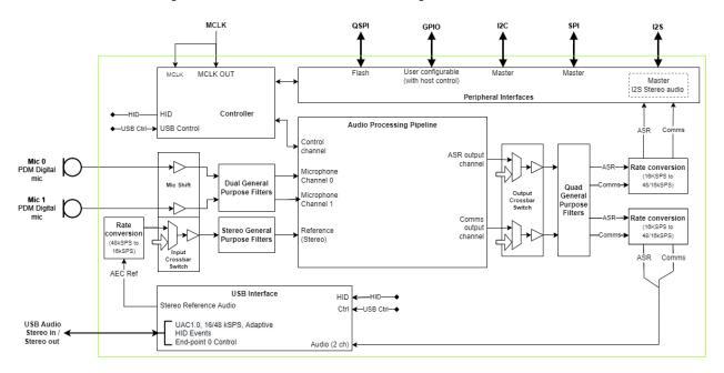
Fig. 1.1: Functional block diagram of XVF3610 in UA configuration
