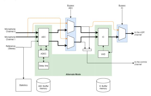
Fig. 2.8: Audio pipeline configuration, [ALT\_ARCH=0] mode
