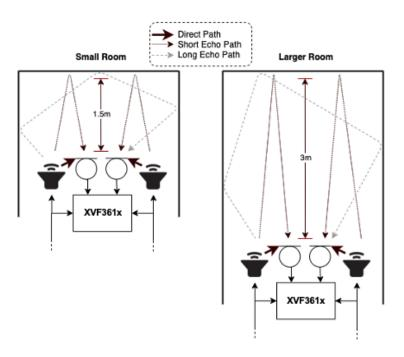
Fig. 2.4: Echo paths from the speakers to the microphones
