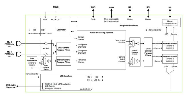
Fig. 1.2: Functional block diagram of XVF3610 in UA-HYBRID configuration
