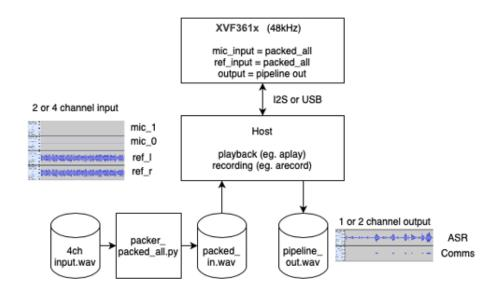
Fig. 7.6: System overview to inject a four-channel, 16kHz test vector into the DSP pipeline
