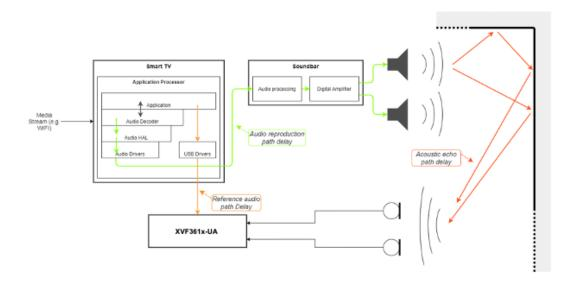
Fig. 2.6: ADEC use case diagram
