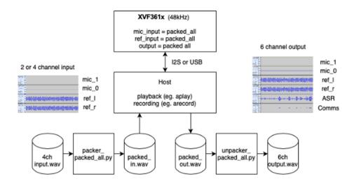
Fig. 7.7: System overview to inject a four-channel packed input and capture a six-channel packed output
