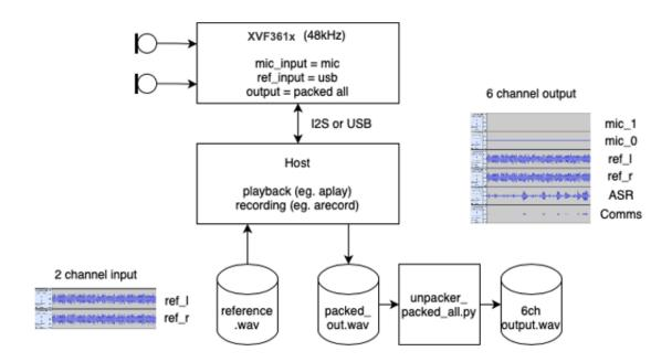
Fig. 7.4: System overview to capture of DSP pipeline signals over a 48kHz USB interface
