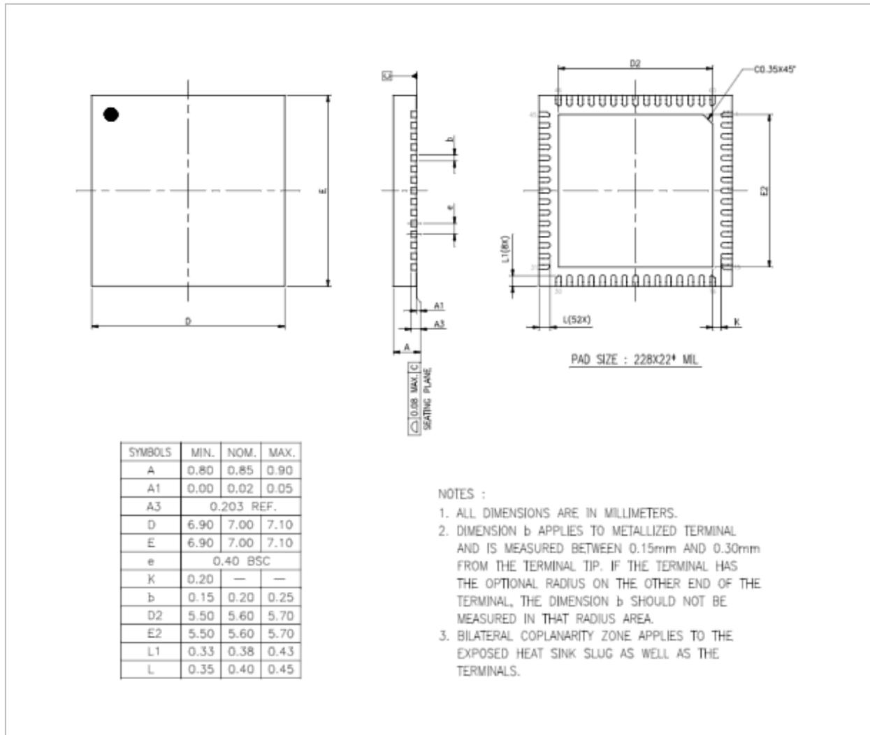
Figure 8-1 QFN60 package dimensions
