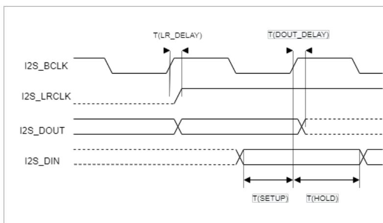
Figure 6-2 I2S master timing
