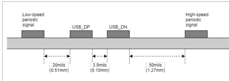
Figure 7-1 USB trace separation showing low speed signal, a differential pair and high-speed clock
