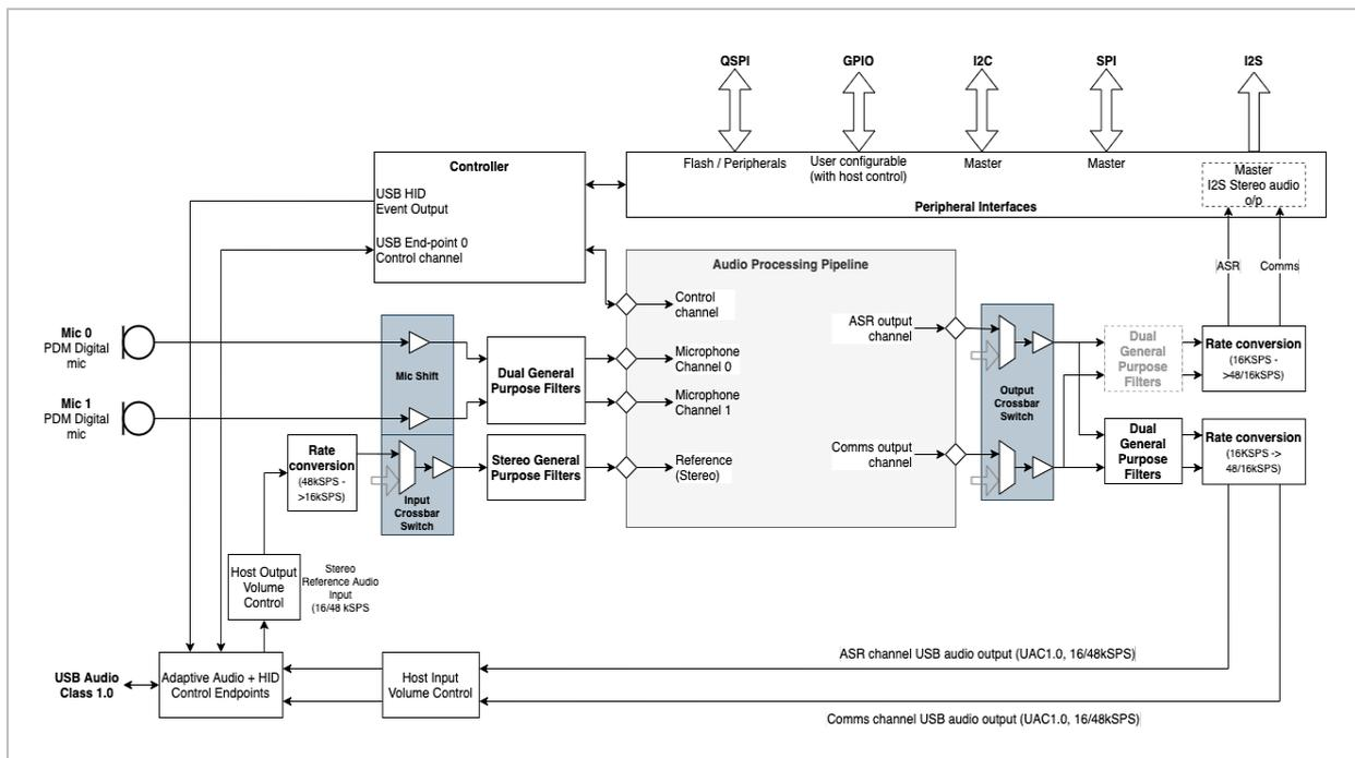
Figure 1-1 Functional block diagram of XVF3510-UA
