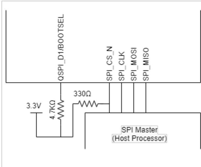
Figure 3-3 XVF3510 SPI slave boot configuration
