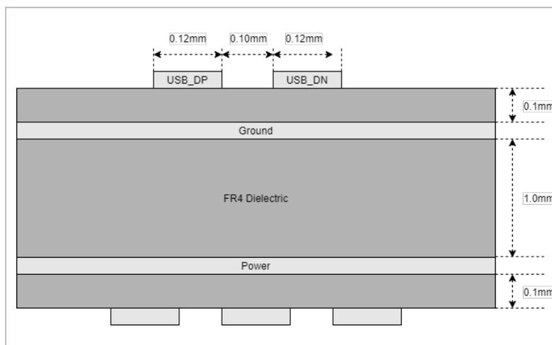
Figure 7-2 Example USB board stack
