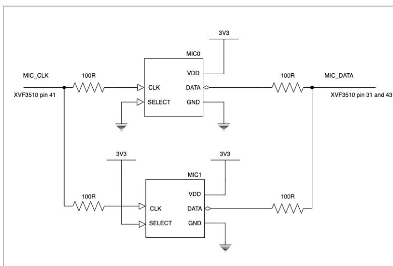
Figure 3-2 PDM microphone schematic
