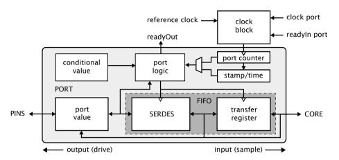
Figure 4: Port block diagram
