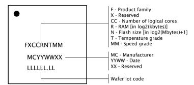
**Figure 29:** Part marking scheme
