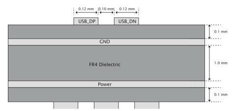
Figure 17: Example USB board stack
