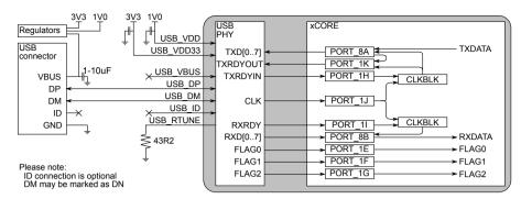
Figure 11: Bus powered USB-device
