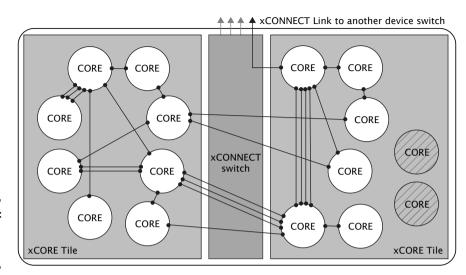
Figure 6: Switch, links and channel ends
