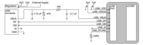
Figure 12: Self powered USB-device
