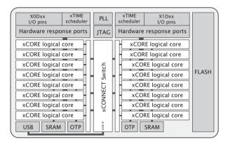
Figure 1: XUF216-256-TQ128 block diagram
