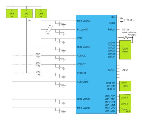
Figure 2: Simplified Reference Schematic
