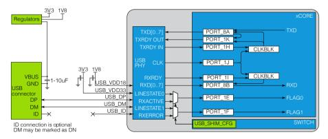
Figure 22: Bus powered USB-device
