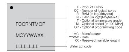
Figure 45: Part marking scheme
