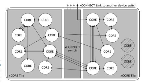
Figure 6: Switch, links and channel ends
