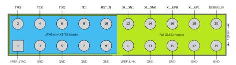
Figure 56: xSYS2 header pin-out, as seen from above
