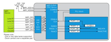
Figure 24: Connecting a MIPI-device
