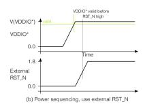
Figure 28: Sequencing of power supplies and RST\_N (if used)
