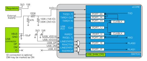
Figure 23: Self powered USB-device
