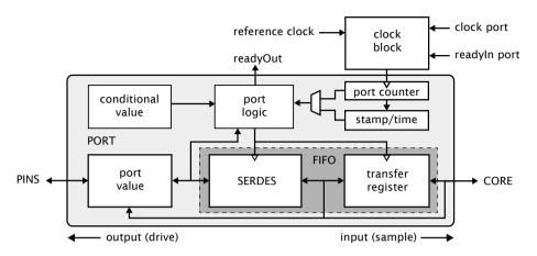
Figure 4: Port block diagram
