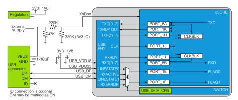
Figure 23: Self powered USB-device
