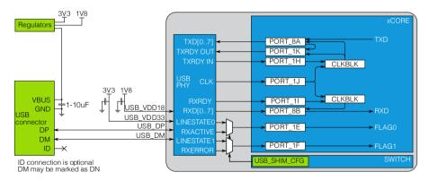
Figure 22: Bus powered USB-device
