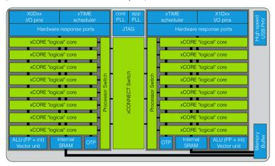
Figure 1: XU316-1024-QF60B block diagram
