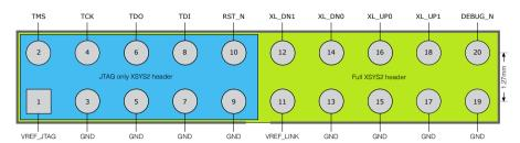
Figure 52: xSYS2 header pin-out, as seen from above
