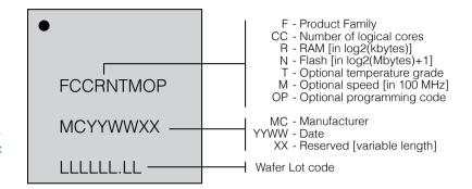
Figure 42: Part marking scheme
