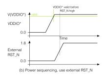
Figure 27: Sequencing of power supplies and RST\_N (if used)
