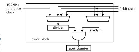
Figure 5: Clock block diagram
