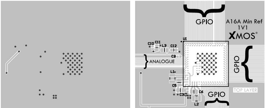
Figure 20: Example minimal system schematic, with top and bottom layout of a 2-layer PCB
