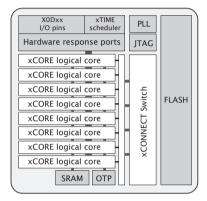
Figure 1: XLF208-256-TQ64 block diagram
