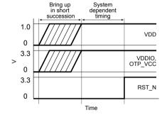
Figure 14: Sequencing of power supplies and RST\_N
