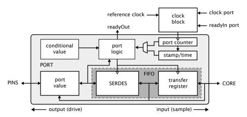
Figure 4: Port block diagram
