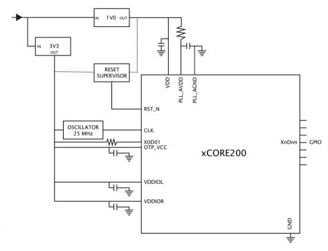
Figure 2: Simplified Reference Schematic
