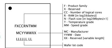
Figure 26: Part marking scheme
