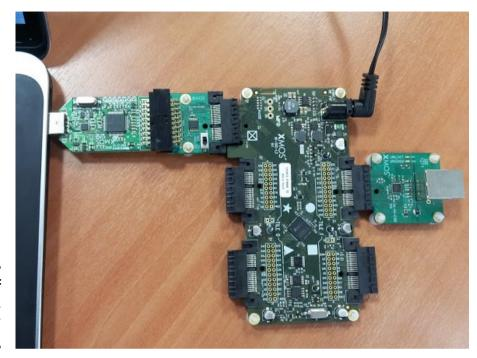
Figure 1: Hardware Setup for Simple HTTP Demo
