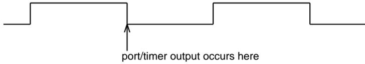
Before returning to the main loop, update the timer output to happen after the next port output (note that the timer and port are running of the same underlying clock):
