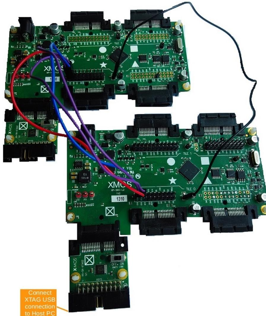
Figure 3: 2-wire XMOS xCORE-L16 sliceKIT set up for off-chip xCONNECT communication
