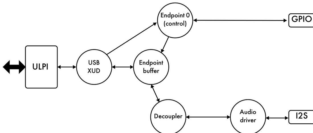
Figure 1: L1 USB Audio Software Core Diagram
