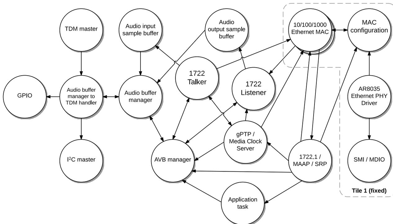
Figure 2: Task diagram of the AVB endpoint example
