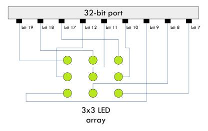
Figure 1: startKIT LED port connection
