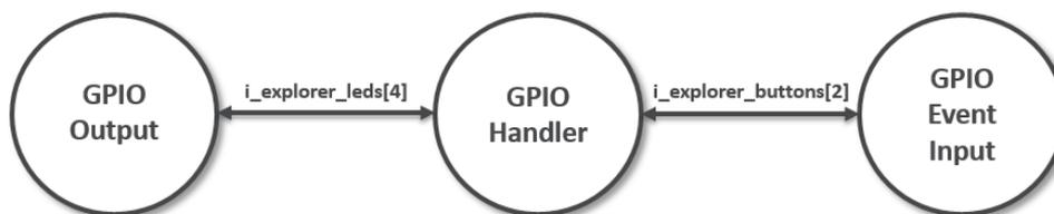
Figure 2: Task diagram of simple GPIO example
