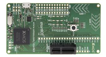
Figure 1: XMOS startKIT core module board setup
