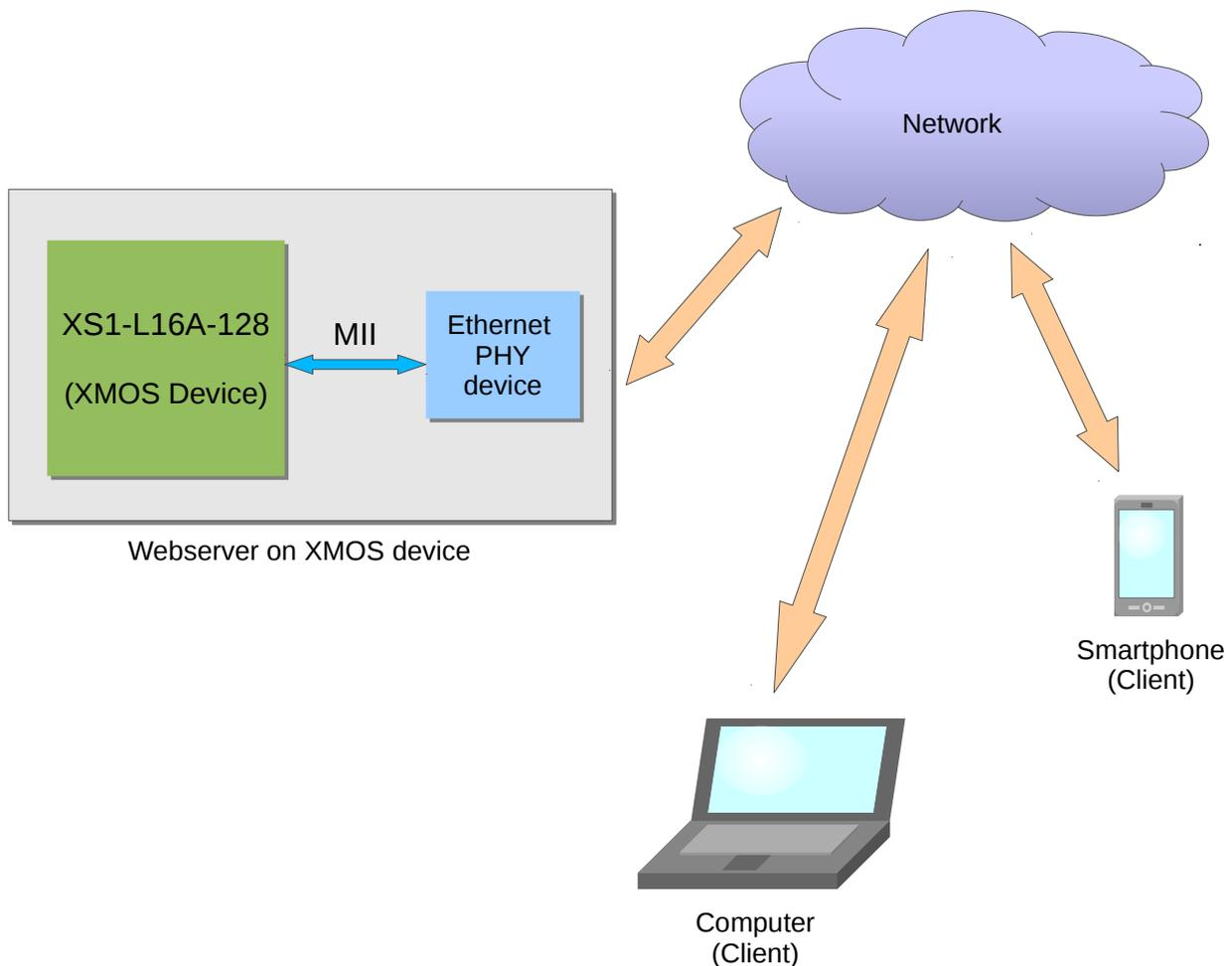
Figure 1: Block diagram of Embedded Webserver example
