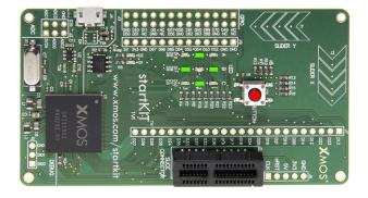
Figure 3: XMOS startKIT core module button down boot
